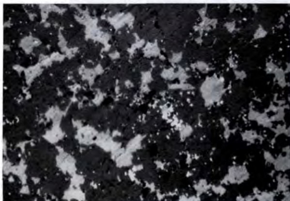
Fig. 5. Sphalerite-dolomite mineralization represented by dolomite rhombohedral crystals and fine-grained sphalerite metasomatically replacing the limestones. Along the borders of the two minerals there are pyrite-bravoite aggregates. Scale 63:1
