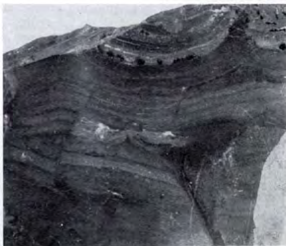
Fig. 3. Banded texture (case 3) in massive metasomatic sphalerite. Galena metacrysts developed in some of the bands or as veinlets cutting the bands. Scale 1:1
