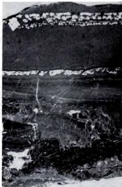
Fig. 2. Banded texture (case 2) of galena-sphalerite mineralization, transitional to brecciated texture. Some of the bands formed by subparallel blind veinlets of galena metacrysts. Scale 10:1
